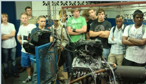
This is the Honda CBR600 engine ready for testing on our engine dynamometer.
